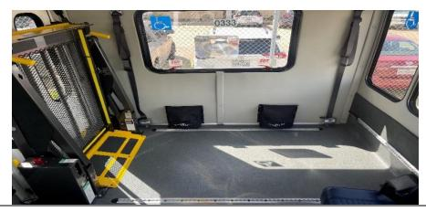
The ramp is manufactured to carry an approximate load capacity of 600LBS (including wheelchair operator and the wheelchair device in use).
